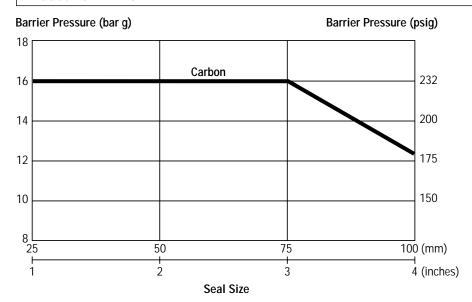
The Basic Pressure Rating is based on a standard seal installed according to the criteria given in this data sheet at a minimum speed of 1450rpm, and according to generally accepted industrial practices.
